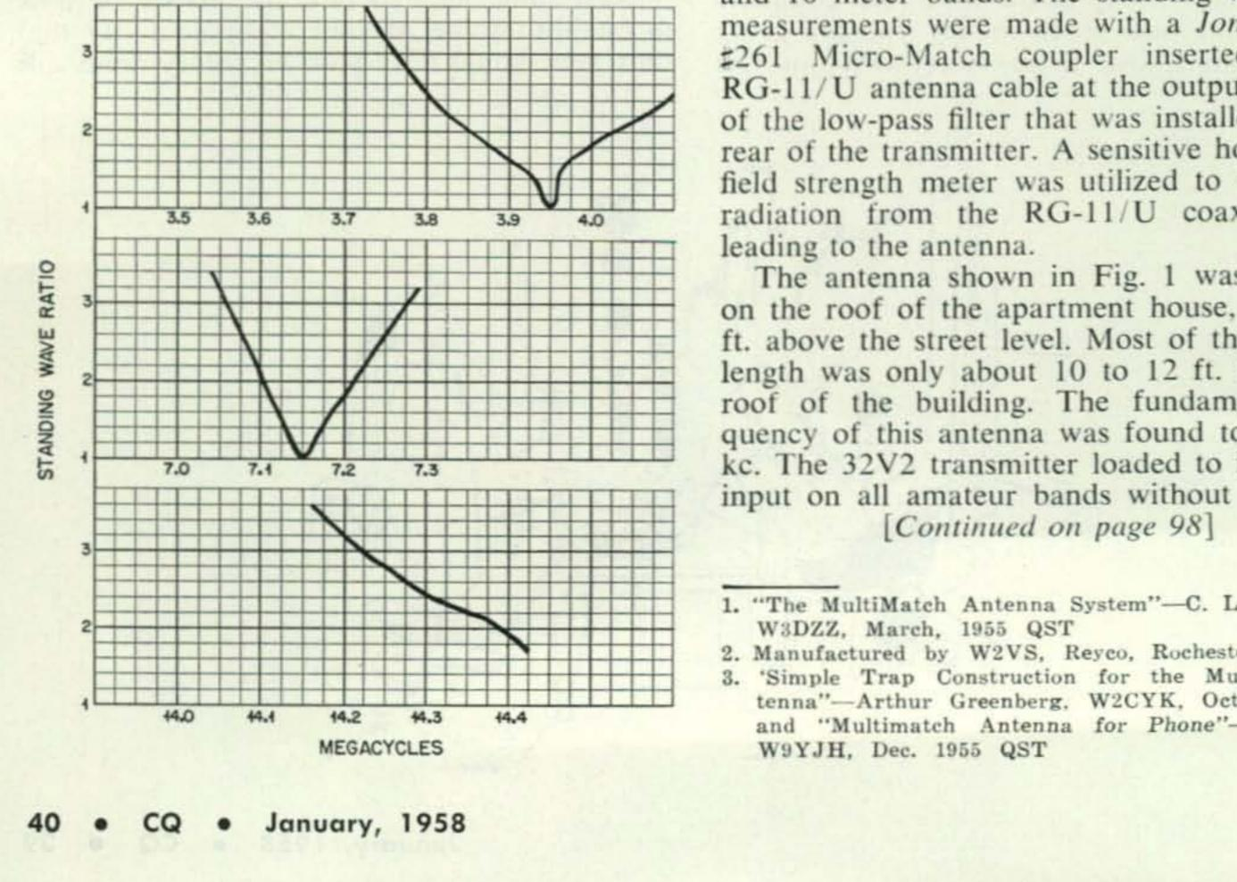
The transmitter used with this multi-band antenna was the Collins type 32V2 which was adjusted for operation in the 80, 40, 20, 15 and 10 meter bands. The standing wave ratio measurements were made with a Jones Model #261 Micro-Match coupler inserted in the RG-11/U antenna cable at the output terminal of the low-pass filter that was installed on the rear of the transmitter. A sensitive home-made field strength meter was utilized to check for radiation from the RG-11/U coaxial cable
